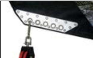
The mainsheet can be hooked into the clew plate in five positions.
